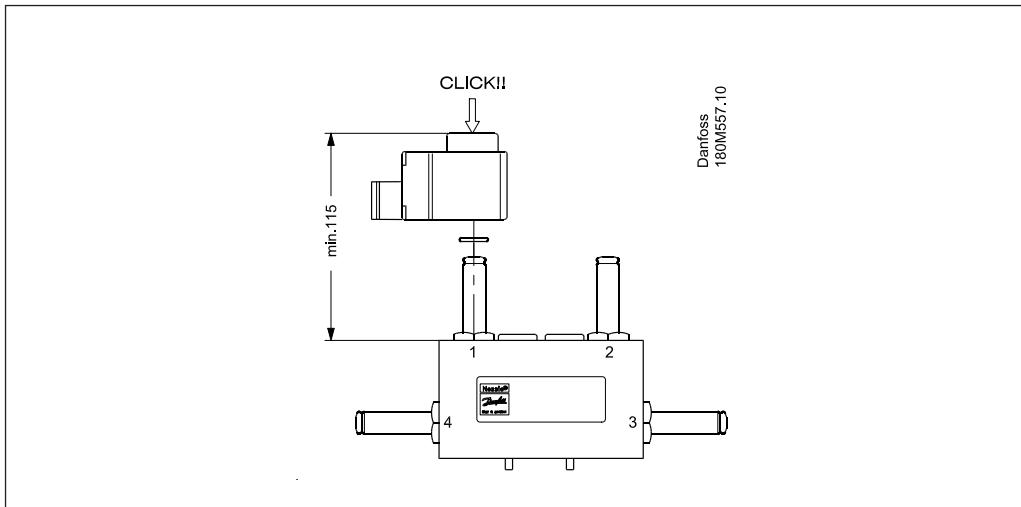
*Coil on valves with short armature tubes (NC and NO valves)*
